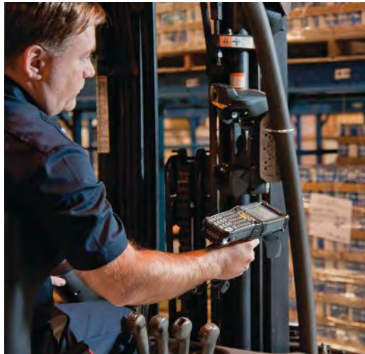
Handheld RFID readers can scan large quantities of items simultaneously in a wide or narrow target field.
