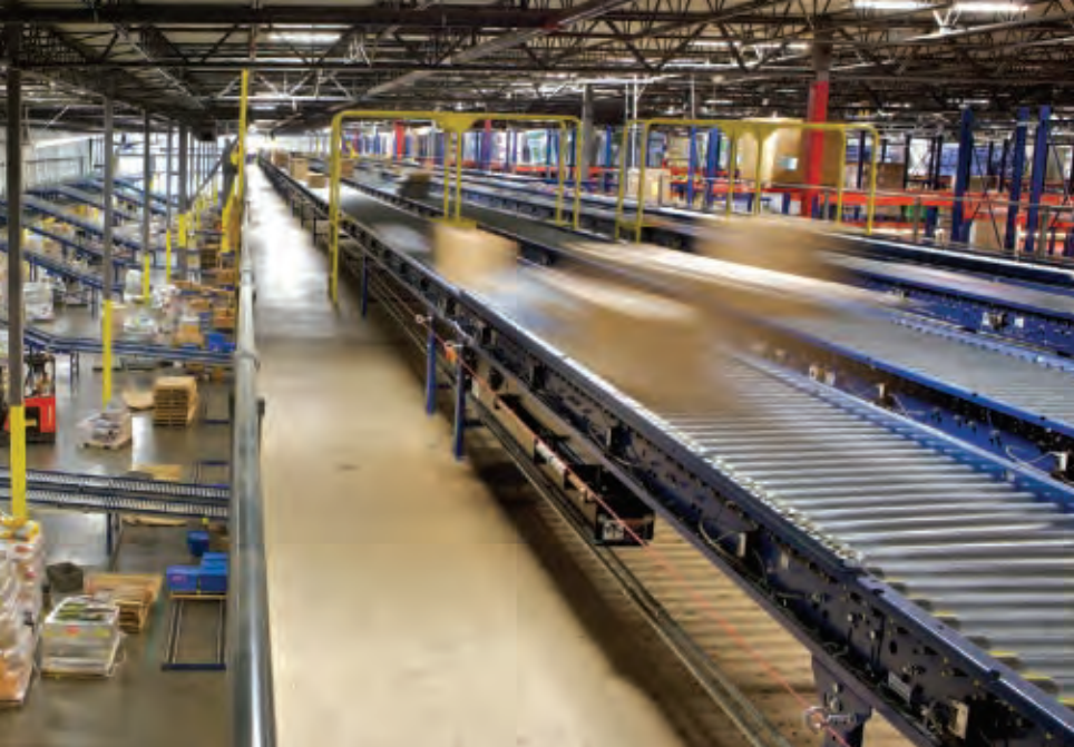
A high speed conveyor and narrow belt shipping sorter handles 120 cartons per minute with mixed sized products.
