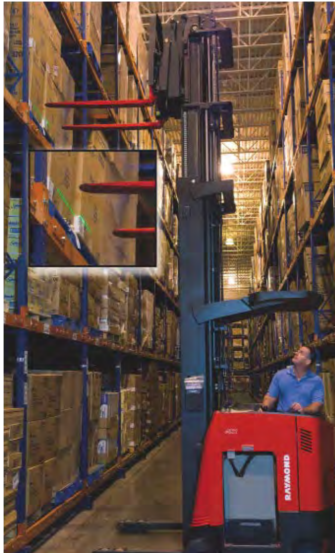
Raymond's fork-tip lasers help reach truck operators accurately engage pallets when storing and retrieving loads, reducing product damage.
